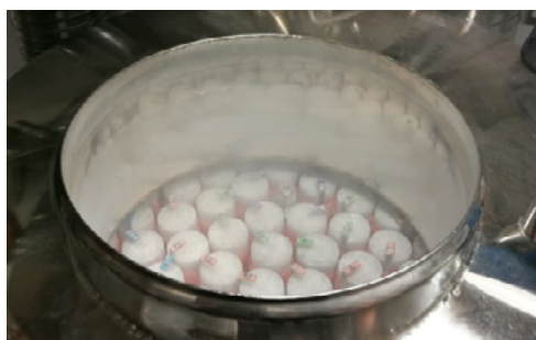
FIGURE 1. Unidentified samples are stored in a freezer, where temperatures can be as low as -200^{\circ}\text{C}
